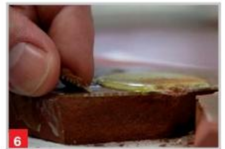
6 ... and the clinker tile breaks! The quality is in the detail. Even after breaking off, the primer is still bonded to the tile. So even if an area became damaged, the damage would not spread.
