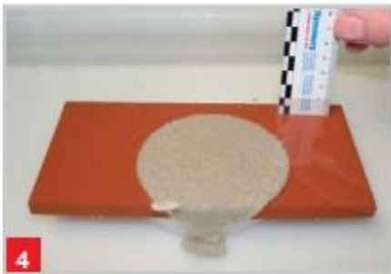
4 Everything runs smoothly: The primer distributes itself evenly and forms a tight bond with the clinker tile.
