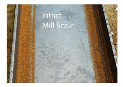
However, when the steel is stored outdoors, the mill scale breaks down and since it is electrochemically cathodic to steel, the steel rusts at the exposed areas.
